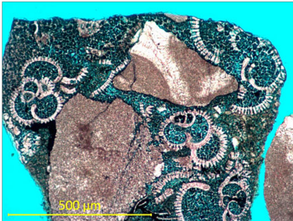
Breccia of Eocene age, offshore Tuxpan Platform. Clasts are of totally cemented up El Abra. The planktonics in the matrix are of Eocene age. Note the ferroan calcite cements (staining blue). Probably this represents collapse of the unstable platform margin into deeper waters during the Eocene. Porosity would have stayed open until deeper burial when the calcite cement occludes all pore space. Photo by Jo Garland . Cambridge Carbonates Ltd.
